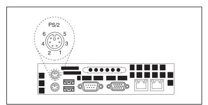
Figure 3-2. PS/2 Connector Location and Pinout
